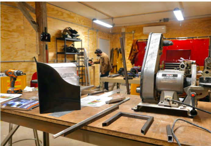
Someone inspects one of the tools in the fully functional metal shop. In the right foreground is a sander that works as a belt sander or a disc sander.
