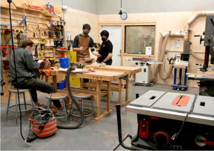
Workers and monitors using equipment in the wood shop, Studio B. Note the ducts on the wall, part of a high-efficiency air filtration system.
